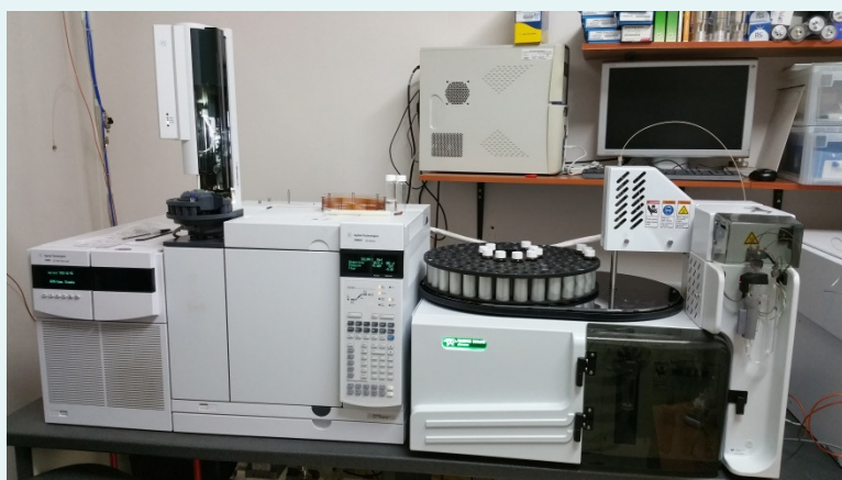
Agilent GC/MS/MS Triplequadrupole Model 7000B and Purge and Trap Atomix Determination VOC Epa 8260
